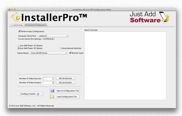
To proceed to the next step in the configuration, click on the Set Up Sources button in the software. A new window will then open that looks as below.
