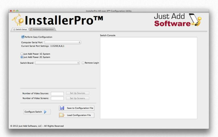
To proceed, first select the desired serial port. Then select if the configuration is being done for a Just Add Power 1G or 2G system. Finally, select the brand of switch being configured. The serial port baud rate will automatically adjust depending on the switch selected. If the standard baud rate needs to be overridden, it can be changed by either clicking on the values after the "Current Serial Port Settings:" label or it can be changed from the edit menu.
