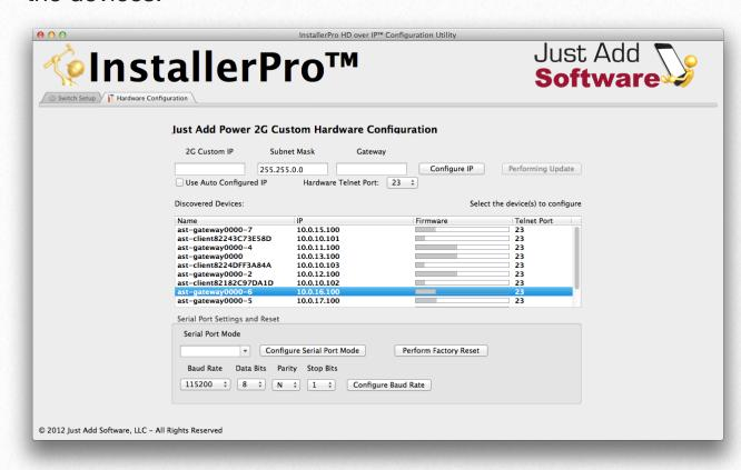
Once all hardware programming is completed, click on the Switch Setup tab to go back to the switch utility. Then enter the commands (or re-program the switch) to put all ports back into their proper VLANs.
