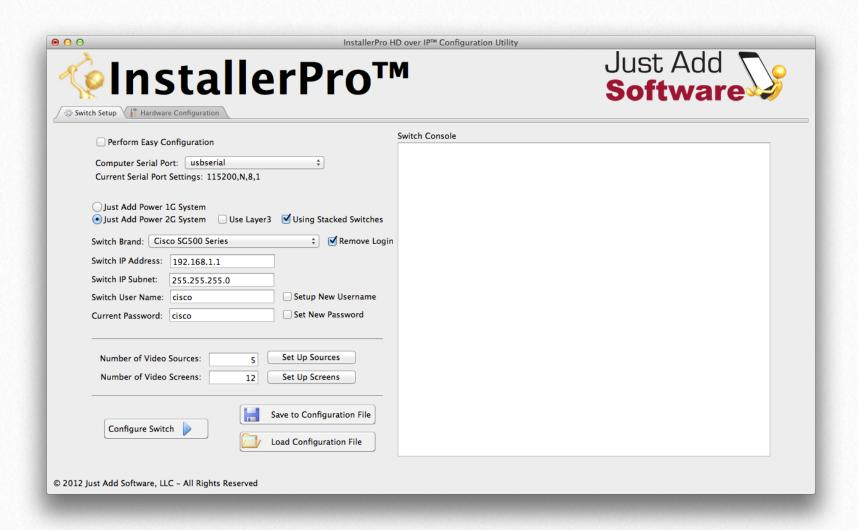
In the example shown, the "Using Stacked Switches" option is selected. If a **stacked switch** configuration is being used, be sure to check this so that the proper stack numbers can be specified when assigning ports to the transmitters and receivers.
