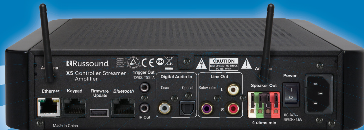
Rusound X5 wireless streamer / controller / amplifier
